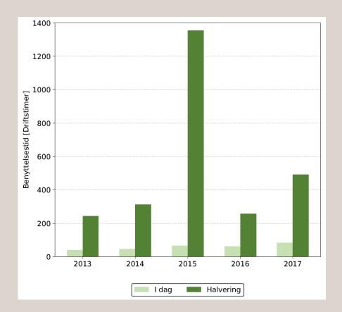
The analysis from 2018 shows that halfing the tariffs would have incresed the production from the electric boilers
